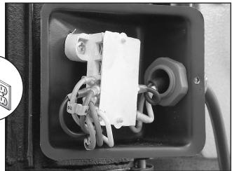
Figure 46. Motor wiring inside junction box.
